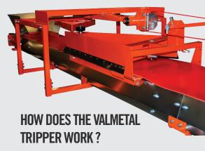
The plow, at every complete revolution, contacts the tripper and changes from one side to the other allowing to feed the opposite side of the conveyor.
